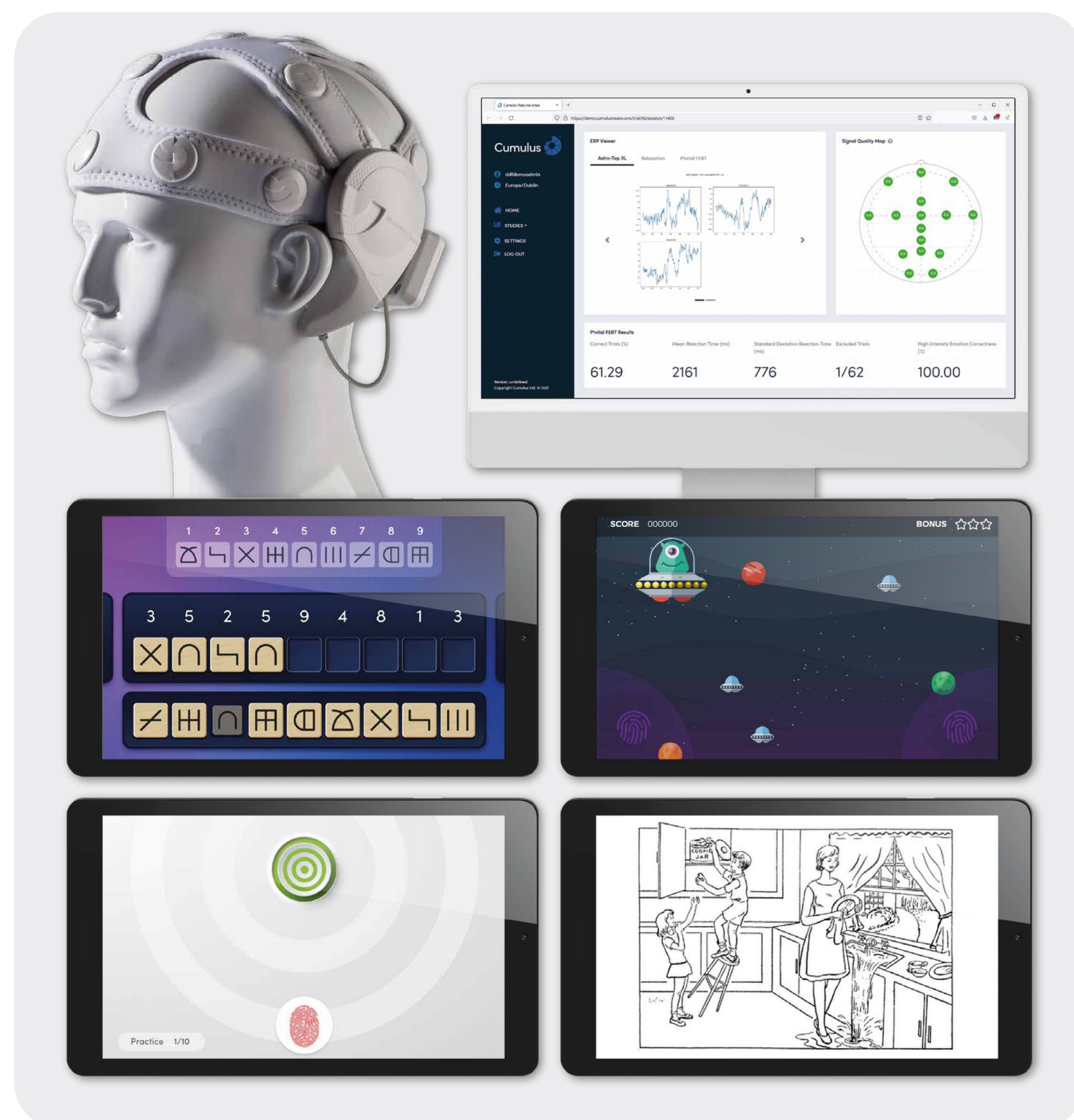
Fig 1. The Cumulus platform. From left to right, Top row: The Cumulus 16-channel dry EEG headset and the online dashboard for remote study monitoring. Middle row: Screenshots of the gamified Digit Symbol Substitution and Oddball tasks. Bottom row: Screenshots of the Psychomotor and Language & Speech tasks.
