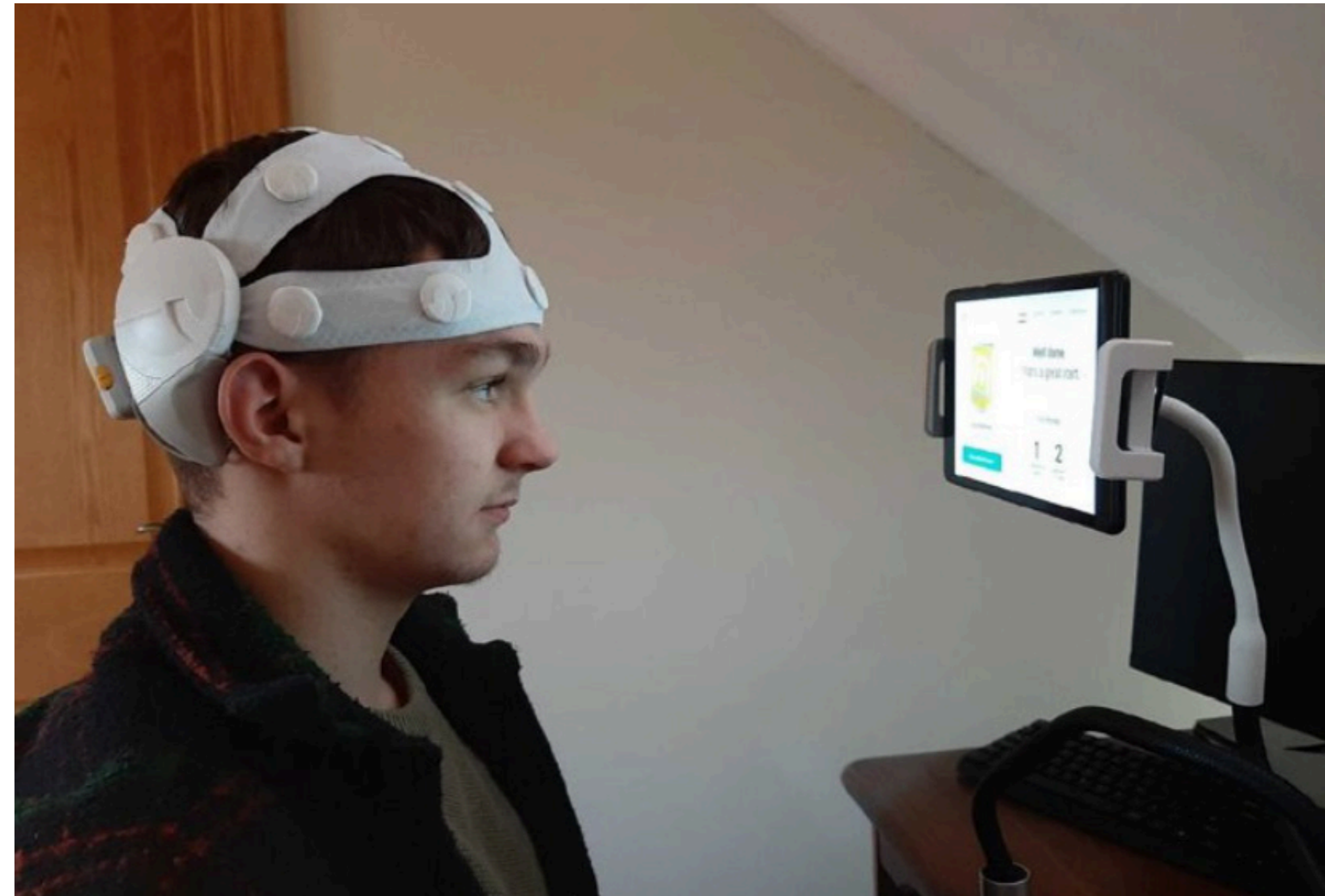
Fig 1. Illustration of set-up using Cumulus 16-channel dry EEG headset, tablet and tablet stand.
